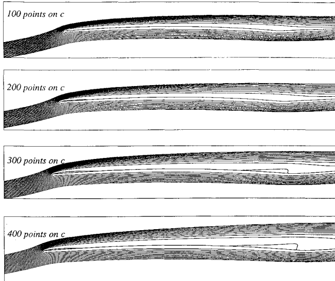
Fig. 4 Effect of grid refinement on stream function contours for a rigid, 2% camber, zero thickness, circular arc airfoil at \alpha = 5 deg and Rn = 4 \times 10^3 .
